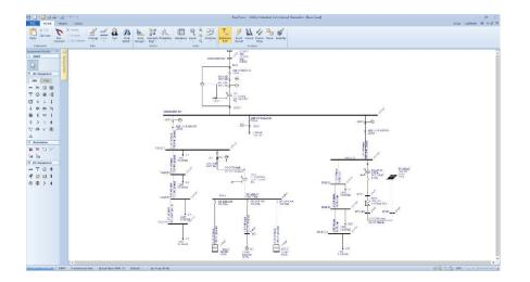
EasyPower's intuitive interface empowers users to digitize their electrical systems, and enables design, analysis, and optimization of complex electrical power distribution systems. *Image courtesy of Bentley Systems*.
