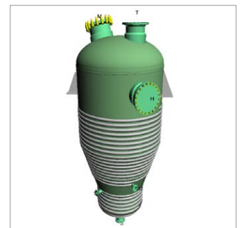
Vessel with limpet coils.
