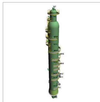
Vertical pressure vessel with platforms and staircase.
