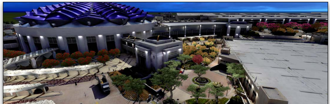
Khatib & Alami captured 330,000 images with UAVs and constructed a 3D reality model of the area, which included 43,000 fully textured buildings.
