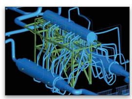
Piping and framework models allow a more accurate understanding of the behavior of frameworks that are connected to piping supports.
