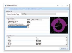
Section properties for built-up sections auto-calculate.
