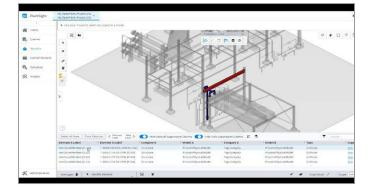
Clash detection helps to increase the accuracy of your design across 3D piping, structures, equipment, and electrical and HVAC systems.
