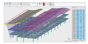
Physical modeling capabilities enable engineers to improve participation in BIM workflows, automatically generating the analysis models for both simple and complex structural analysis.
