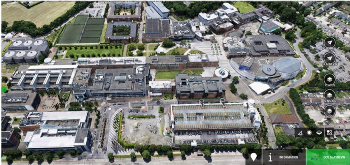
Figure 4: Drone-generated reality mesh of DCU's Glasnevin campus. This was processed using Bentley's iTwin Capture Modeler, providing a detailed and georeferenced base layer for further integration
