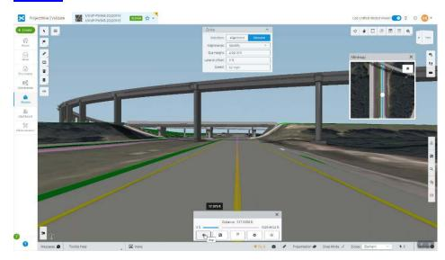
ProjectWise, powered by iTwin, supports full digital delivery, including simulating vehicle drive paths to ensure proper sight lines. *Image courtesy of Bentley Systems*.
