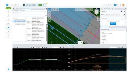
ProjectWise, powered by iTwin, supports full digital delivery including independent roadway corridor super elevation analysis, improving vehicle safety on the resulting roadway. *Image courtesy of Bentley Systems*.
