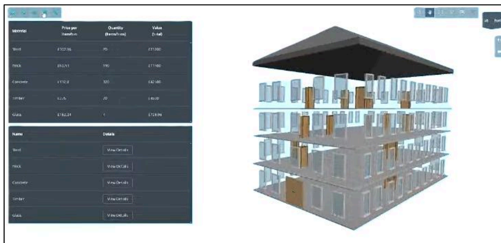
Caption: SiTESalvage's project uses digital twins to transform buildings scheduled for demolition into "resource banks" by digitally mapping their salvageable materials. (Image courtesy of Bentley Systems and Enactus)
