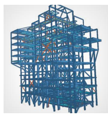
Located in Japan, this project involves structural design of boiler stands for a paper mill. The weight of the machine is heavy, and the structure is complicated. The company delivering this project previously designed boiler stands for nine other projects using software that made it difficult to perform accurate stress analysis. They realized that they needed a robust structural modeling and analysis solution.
