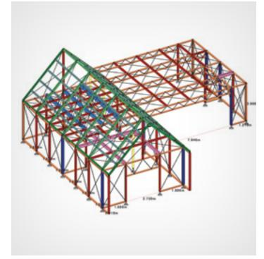
This project involved providing a rational economic design while ensuring structural integrity for approval of a building. The special shape of the lightweight steel structure presented challenges verifying the stress state and determining a cost-efficient design. Existing software applications lacked automation, comprehensive analysis, and structural calculation features.
