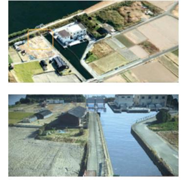
This project was initiated to enable the client, Hamamatsu City, to visualize the river entry and exit along with the newly constructed drainage facility located amid houses in the vicinity. The project team needed to survey and model the existing area and drainage plant and create a digital twin for the client to visualize and assess the layout of the drainage plant.
