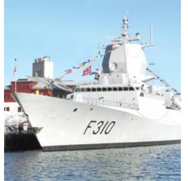
Known as F-310, Fridtjof Nansen is a class of Spanish-made anti-aircraft frigates used by the royal Norwegian Navy, equipped with an advanced combat system capable of detecting aircraft movement within a radius of 500 kilometers. Consisting of five frigates, the program was designed and built at Navantia shipyards through their integrated modular construction (IMC) concept, requiring the implementation of a collaborative modeling platform and connected digital environment.
