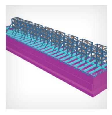
This project involved designing facilities for a combined cycle cogeneration power plant. The scope of work included detailed design, layout, and provision of a calculation report for the superstructure and retention pit. Faced with a confined space and managing large amounts of piping, electrical, and storm water data, the team needed structural design and analysis software to model and assess the reinforced concrete foundation structure and steel superstructure.
