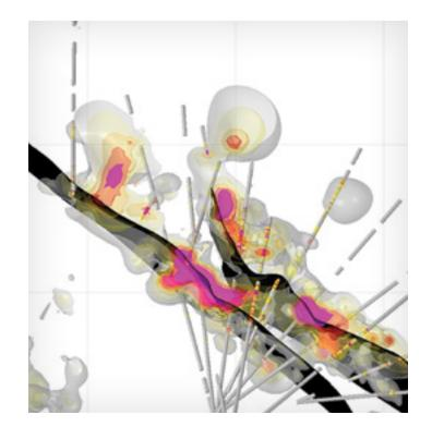
Cerro Lindo is a world-class volcanogenic massive sulfide deposit with an average production of 21,500 metric tons per day. To help identify the possible mineralization directions in the mine, the team initiated a modeling project based on metal ratios and dynamic anisotropy points. Given the irregular shape of certain bodies present in the deposit, traditional explicit modeling processes were not capable of adequately representing the interpolations made by the geology team.
