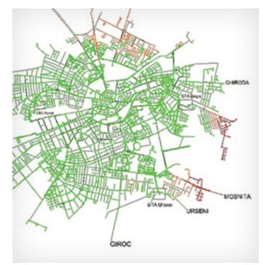
Aquatim SA was tasked with stepping up its hydraulic modeling for the water distribution network in Timișoara, located in western Romania. The USD 200,000 project involved modernizing its digital infrastructure by importing data into a model for easier visibility.
