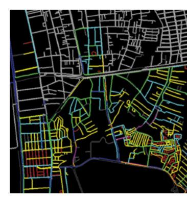
Already familiar with Bentley applications, the team used OpenFlows to analyze the available flow and pressure data and create a simulation. They reduced the potential breakage points to one location, which was confirmed to be the correct location after a physical inspection. The team was then able to inform residents ahead of time to stock up on water ahead of the repair. OpenFlows reduced work hours in the field by 80% and saved PHP 9.88 million in inspection, repair, and fieldwork.
