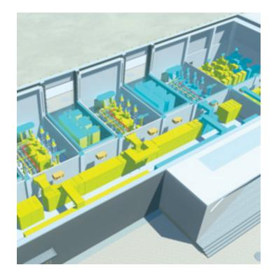
Located in Cangzhou, the Weizhuang 110-kilovolt substation features two main and two grounding transformers, two 110-kilovolt and 14 10-kilovolt outgoing cable lines, and four sets of capacitors. The project presented complex terrain and surrounding structures that needed to be considered in the design to ensure safety and reliability of the plant. To address these challenges, the team needed an integrated digital substation technology solution.
