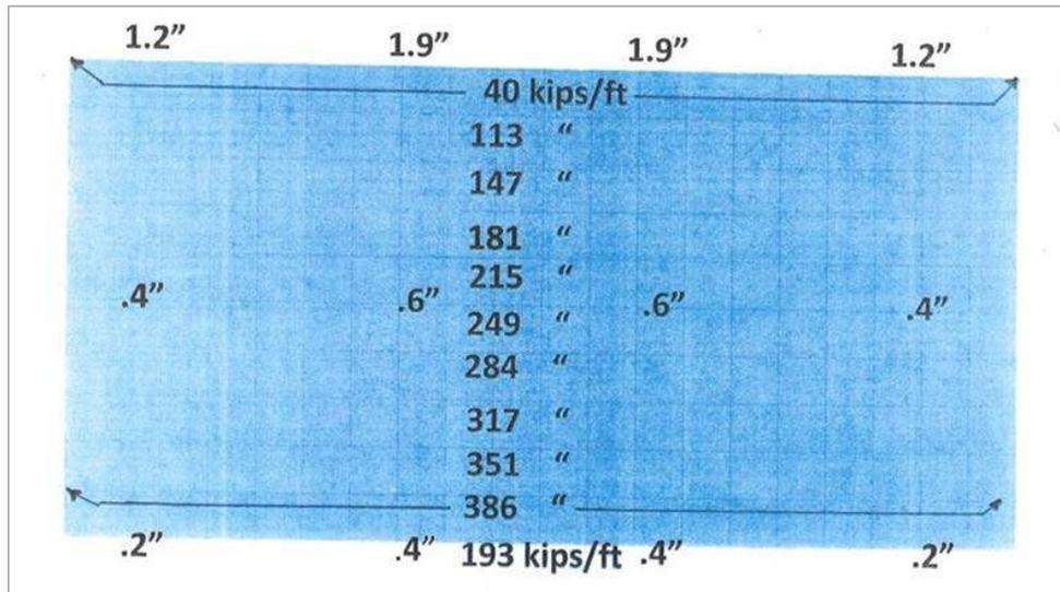
Figure 2 – Final distribution of nodal soil springs.
