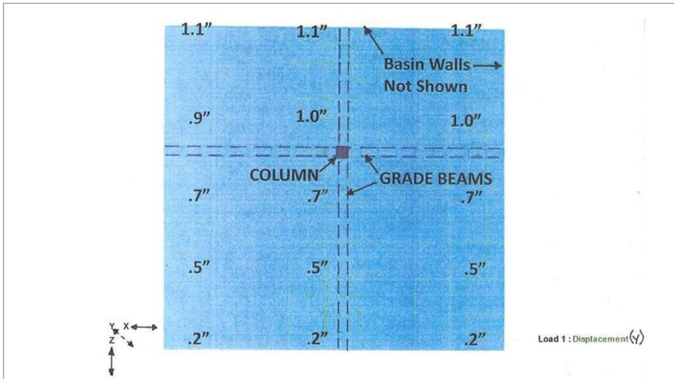
Figure 6 – Beams intersect under the single interior roof support column.
