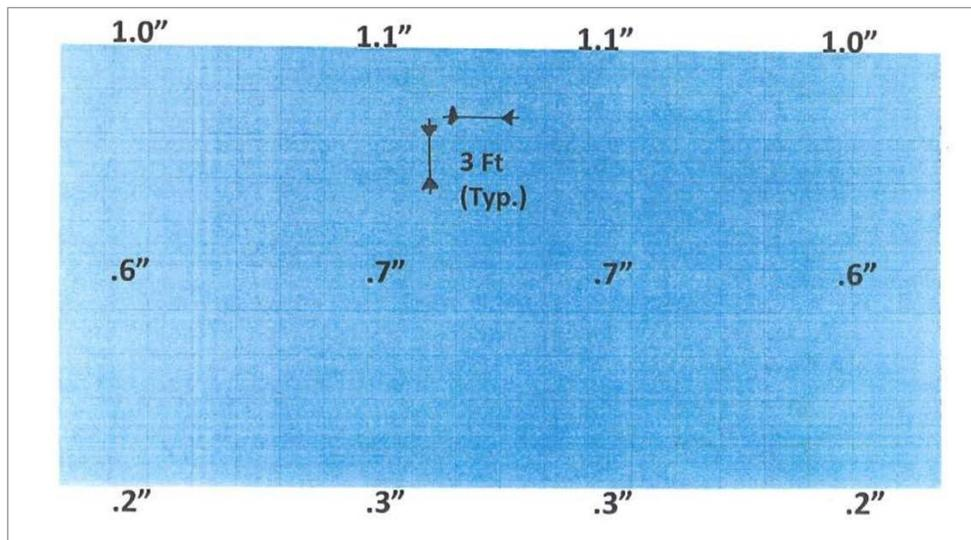
Figure 3 – Mat thickness for acceptable settlement.
